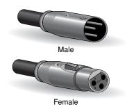
This type of connector is generally referred to as "XLRtype," and almost always carries a balanced signal. If the corresponding circuitry is designed properly, however, XLR- type connectors will also handle unbalanced signals with no problem. Microphone cables usually have this type of connector, as do the inputs and outputs of most professional audio gear.
