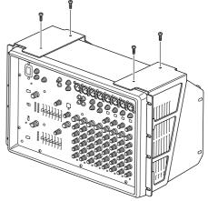
■ How to install the rack-mount hardware
