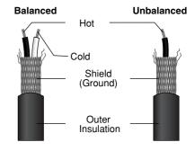
While the desired audio signals in the hot and cold conductors are out of phase, any noise induced in the line will be exactly the same in both conductors, and thus in phase. The trick is that the phase of one signal is reversed at the receiving end of the line so that the desired audio signals become in-phase, and the induced noise suddenly finds itself out of phase. The out-of-phase noise signal is effectively canceled while the audio signal is left intact. Clever, eh?
