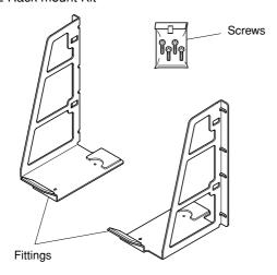
2 Using the kit's 4 screws, attach the kit's 2 metal fittings as shown below.
